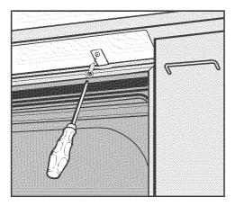
Using flat head screws, secure the dishwasher to the countertop by screwing through both the mounting bracket and the steam deflector. Make certain that the white rubber seal located at the top, outer edge of the dishwasher is tight against the bottom of the countertop. Do not drill any additional holes through the wash cabinet. If in doubt on how to secure the dishwasher, please call Miele's Technical Service Department. For openings exactly 23  $^{5}\!/_{8}$  " (60 cm) wide:
